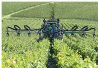
*Easyflo is a new calibration module for pneumatic vineyard sprayers for improved precision and spray output distribution. Easyflo allows for the application of very low volumes per hectare with no risk of clogging combined with an ability to shut down spraying by rows or half rows to prevent dispersion outside the desired treatment area. This capability results in a 15% reduction in the volume of pesticides sprayed.*
