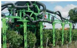
*Précijet is an interlined system for spraying in vineyard rows for optimal local application according to the volume of vegetation. This makes it possible to avoid overdosing amounts starting with the first treatment of the season when vegetation is still not dense. In this way Précijet makes it possible to reduce the quantities of pesticides sprayed by 30%.*
