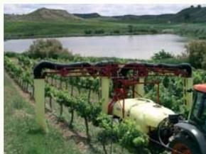
*The IRIS application system uses an air-assisted spraying technology, for precision targeting the droplets dispersed to cover the entire plant improving penetration deep in the foliage. This in turn considerably reduces both drift and product consumption. The IRIS system was awarded a prize for innovation at FIMA 2010, Spain's major International Fair of Agricultural Machinery.*
